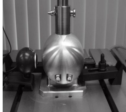
Image of test set-up used for compression-shear testing according to ASTM F2077
